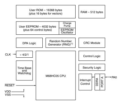
Note: 1. A sampling/smoothing algorithm MUST be used in conjunction with the RNG to obtain statistically random results across all operating conditions.
